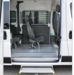
Electric step and handle on the side entry provide easy access to the passenger compartment.
